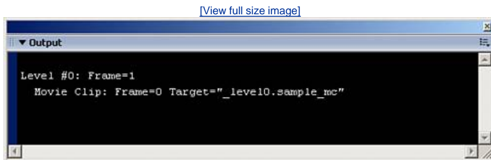
Figure 13.1. Using the List Objects option under Debug, you can see the movie clip you created via ActionScript.
