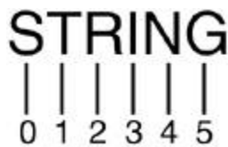
Figure 9.1. Indexing strings start with index 0 for the first character.
